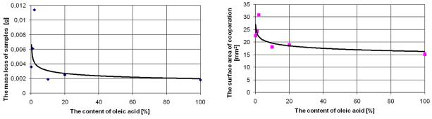
Fig. 2. Summary of the results of the lubricating properties of rapeseed oil methyl esters with addition of oleic acid according to [15]
