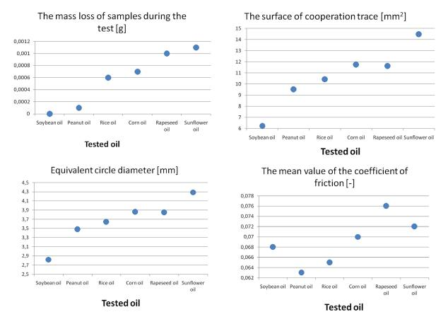
Fig. 1. Summary of the results of the lubricating properties of vegetable oils tested
